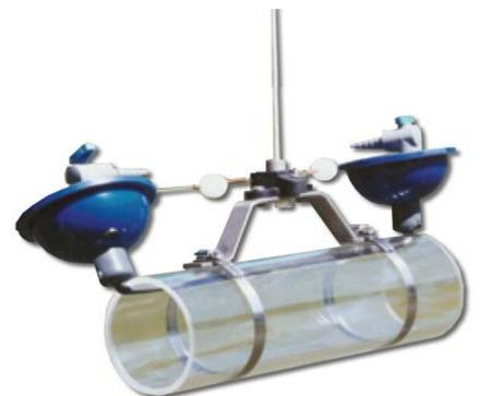
The Van Dorn sampler is a clear cylinder shaped container about four inches in diameter and about a foot long. It is open on each end to allow water to flow through. It has a soft rubber ball at each
